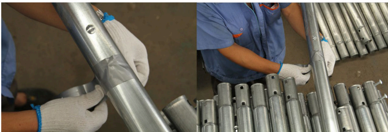
Wrapping the structure joints with tape
